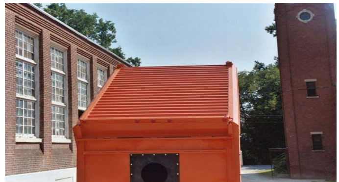
Corrugated Steel Top to Aid in Directing Air Flow - Down Draft
