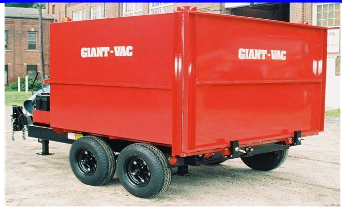
Top Hinged Full Width Doors for Ease in Dumping
