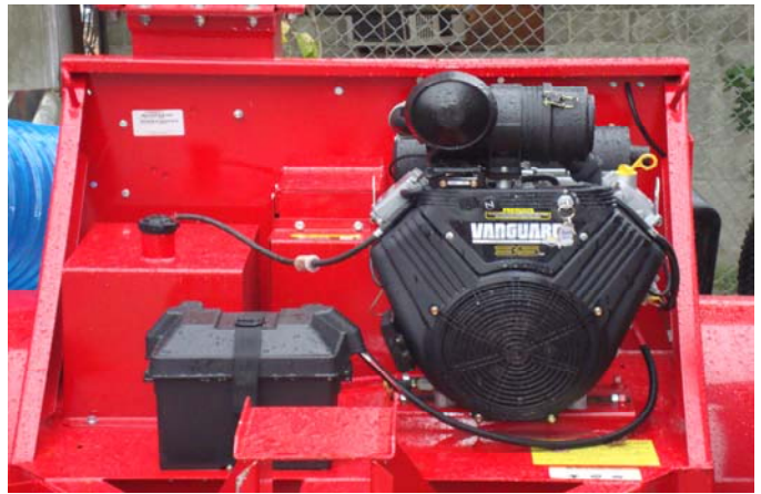
35hp V-Twin Engine & Weather-Proof Battery Box
