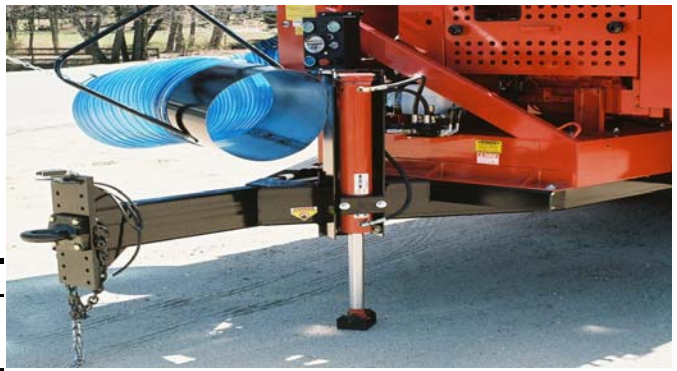
Adjustable Tow Tongue with Hydraulic Jack
