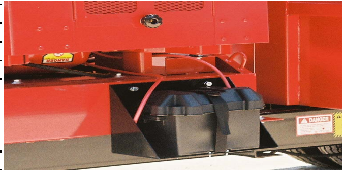
Covered Battery Box
