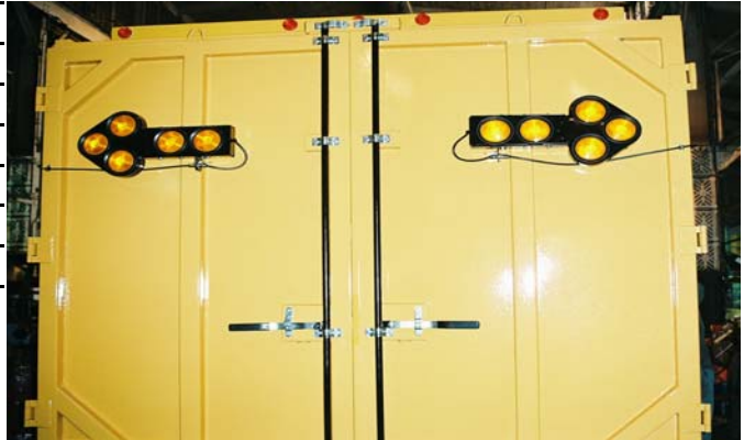
Barn-Type Rear Doors with Two-Piece Arrow Boards
